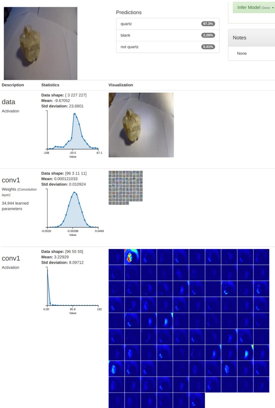
Figure 11: test image shows correct classification of a yellow-ish quartz
